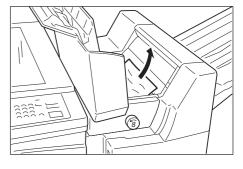
If the jammed paper could not be removed easily, turn Knob 8 counter-clockwise to eject the paper.
